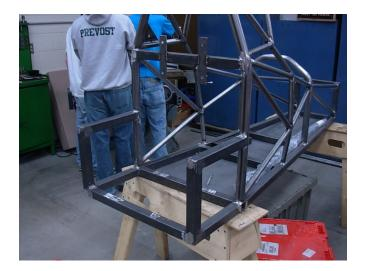
Our chassis with the pieces of flat bar welded to it.
